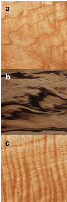
A few patterns of figured wood: a. curly big leaf maple, b. spalted white oak, c. quilted big leaf maple. Photos courtesy of North Woods LLC.
